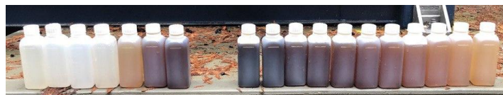
Figure 14 Regeneration waste's colour change after the IEX 301 regeneration (October 26, 2020)
